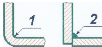
Figure 3. Permissible values of Food Zone radii: 1) radius when processed with a cutting tool - not less than 3.2 mm; 2) radius of the welded seam - not less than 3.2 mm – adopted from [18]
