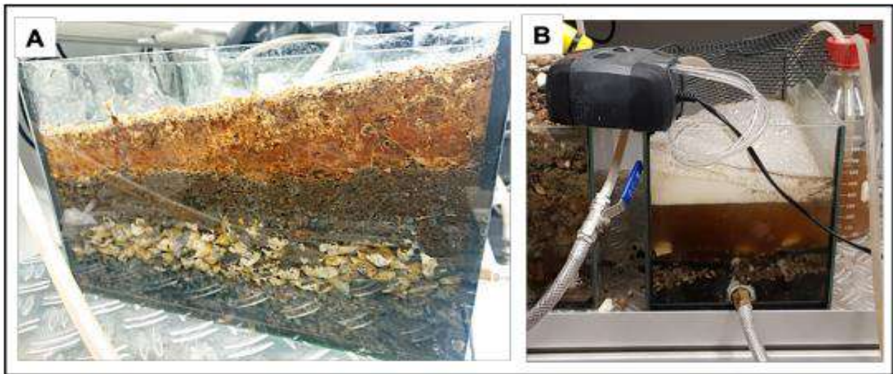
Figure 4. Images of the laboratory scale wetlands (operating at Partner 2 – UW on a regular basis) aimed to carry out manipulative experiments in WP5. (A) The layered configuration of the system. (B) Peristaltic pump operating in the system. The UW's know-how concerning this lab-scale CWs will be transferred internally to other partners involved in the project.
