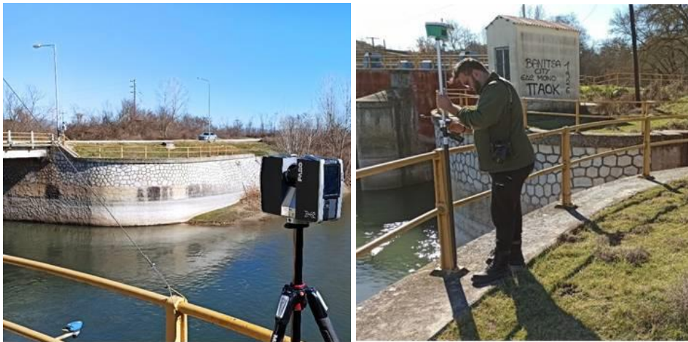
Fig. 3. left) The Faro Focus X130 laser scanner and right) topographic measurements of the control points – georeferencing via the GNSS RTK receiver.
