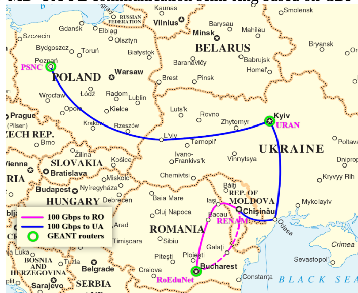
Fig. 1. RO-MD-UA-PL communication semi-ring based on CBF connections
